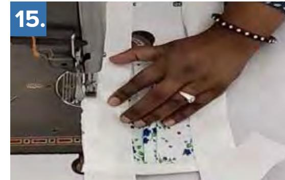
**Now begin attaching the long 40" strips used for tying the face cover to the top and bottom as shown.**
