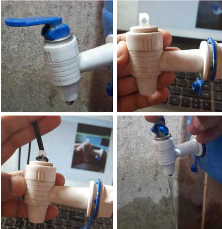
Spring loaded taps that are typically used in water filters can be fitted with a brake wire connected to a pedal
