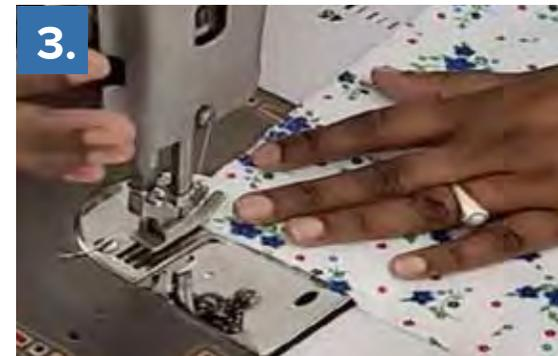
Take the cut fabric, attach the 1.5x5" strip to be used as piping to the fabric on one end as shown.
