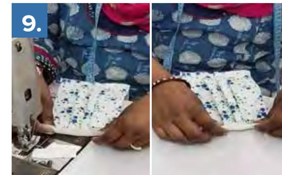
Turn the pleated cloth to the other side and repeat steps for pleating on this side as shown above. Once the pleats have been made, the height of the pleated cloth will be reduced from 9" to 5".
