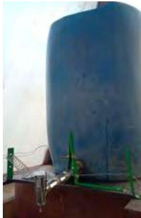
Can use any existing container: up to 20 litre system is recommended along with 2 buckets of 10 litre each that are seated on floor as back up for quick replacement.
